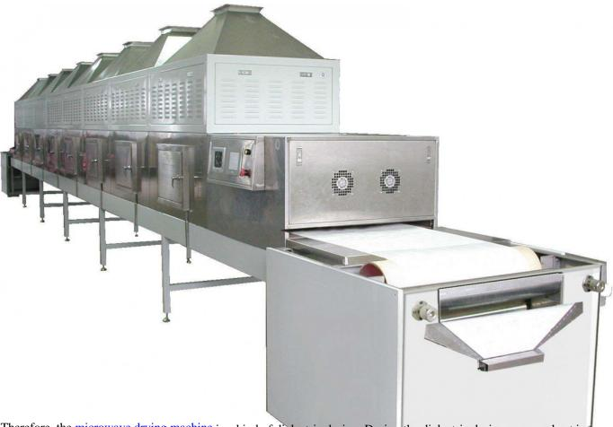
Therefore, the <u>microwave drying machine</u> is a kind of dielectric drying. During the dielectric drying process, heat is generated inside the material, and the mass transfer driving force is mainly a vapor pressure gradient rapidly generated inside the material.
